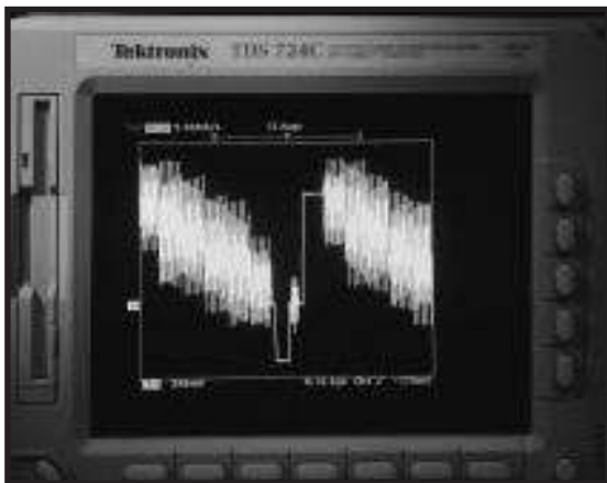
A traditional DSO is unable to display the details and dynamic changes of this composite video waveform.
