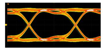
Use the 750 MHz bandwidth and 1.5 GHz bandwidth model respectively to perform eye measurement on the 1 Gb/s signal.
