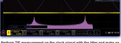
Perform TIE measurement on the clock signal with the jitter and make an analysis on the measurement results through trend graph and histogram.
