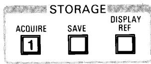
**1. ACQUIRE** starts/restarts the acquisition from SAVE mode. If single seq trigger mode is on, turn it off to gain access to the acquire menu when fast completing sequences are being acquired.
