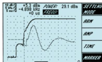
Measurement of power levels upon switching a transmitter on and off or of power ramps (data transmission system)
