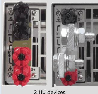
Bigger devices have got solid copper bars with screw terminals. 600 W devices also have terminals at the front.
