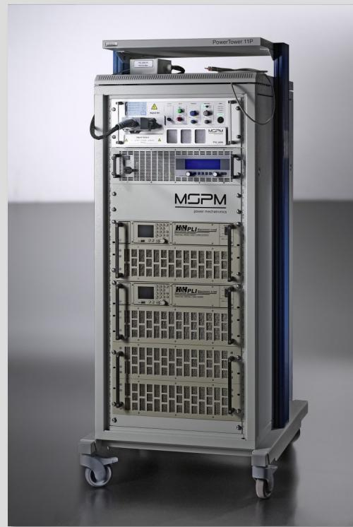
System with PLI4806 and PLI9860 for testing transformers.
