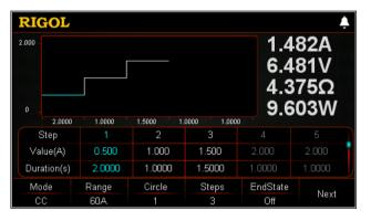
You can generate complex sequences by editing the setting value for each step, the dwell time, and slew rate (the slew rate can only be edited in CC mode) to meet the complex test demands.
