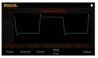
The electronic load provides the waveform display function and supports the following operations for the waveform, such as pausing the waveform, enlarging and narrowing the waveform, and capturing the waveform. Therefore, you can dynamically observe the trend of parameters changes.
